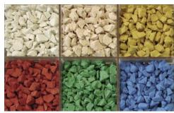
■ Granule. The granule is available in many colours, and produces a 'through and through' surface. A slight discolouration caused by UV rays is possible. The granule is flame proof and, if necessary, can be cleaned under high pressure.
